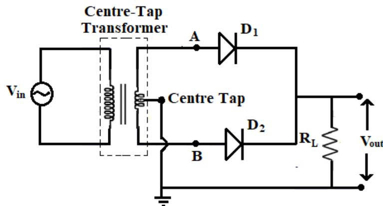
The circuit diagram is as shown in the figure. The diodes D<sub>1</sub> and D<sub>2</sub> with a load resistor R<sub>L</sub> are connected across the secondary of the transformer. The R<sub>L</sub> is connected to the center tap of the secondary transformer. The A.C voltage to be rectified is applied to the primary of the transformer.
