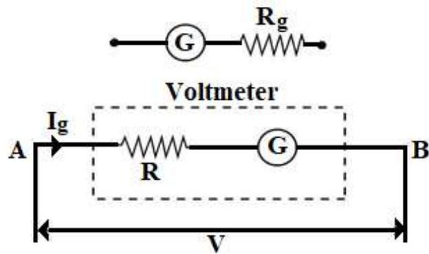
A galvanometer can be converted into a voltmeter by connecting a high resistance in series with the coil of the galvanometer. Let  $R_g$  be the resistance of the galvanometer,  $I_g$  be the current required for full scale deflection and  $R$  be the high resistance to be connected in series with the galvanometer. If  $V$  is the maximum potential difference to be measured then
