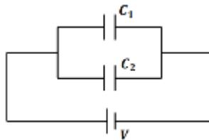
Consider three capacitors of capacitance  $C_1$  and  $C_2$  connected in parallel between A & B as shown.
